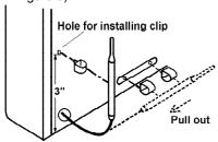
Figure 5 - Moving Thermostat Sensing Bulb
